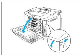
3 Pull out all the toner cartridges from the printer.
