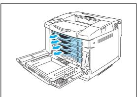
**4** Fit an orange protective cover to each of the toner cartridges.
