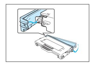
Put the toner cartridge in one of the toner bags, fit a left and right packing material and then put the toner cartridge in the toner box.
