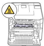
4. Holding the handles on both sides, squeeze the gray levers on the fuser unit and pull downward. Apply downward pressure on the fuser unit and pull it out of the machine.
