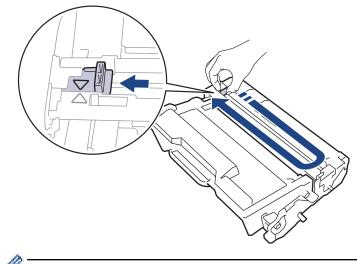
Be sure to return the tab to the Home position ( $\blacktriangle$ ). The arrow on the tab must be aligned with the arrow on the drum unit. If it is not, printed pages may have a vertical stripe.
