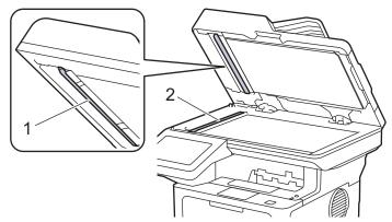
4. (For automatic 2-sided scanning models) Open the scanner glass cover (1), and then clean the other white bar (2) and scanner glass strip (3).
