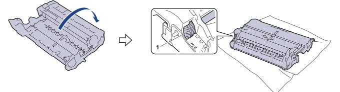
10. Use the numbered markers next to the drum roller to find the mark on the drum. For example, a dot in column 2 on the check sheet means that there is a mark in drum region "2".
