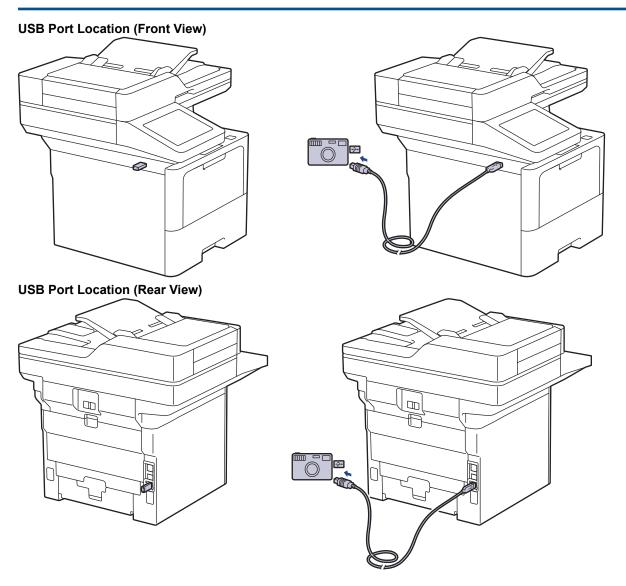
1. Connect your USB flash drive or digital camera to the USB direct interface. The touchscreen will automatically display the USB menu to confirm that the USB flash drive or digital camera is correctly connected.
