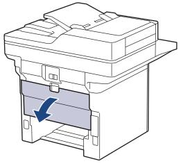
7. Pull the green levers at the left and right sides toward you to release the fuser cover.
