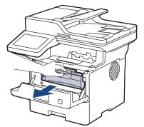
8. Push down the green lock lever and take the toner cartridge out of the drum unit.
