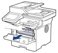
3. Clean the corona wire inside the drum unit by gently sliding the green tab from left to right and right to left several times.
