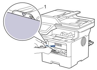
Load the envelopes in the MP tray with the printing surface face up. Make sure the envelopes are below the maximum paper mark (1).
