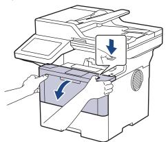
7. Remove the toner cartridge and drum unit assembly from the machine.
