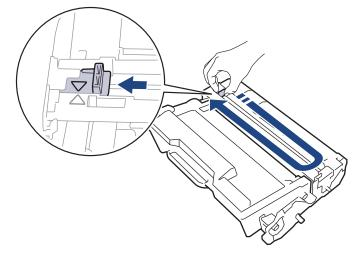
Be sure to return the tab to the Home position ( $\blacktriangle$ ). The arrow on the tab must be aligned with the arrow on the drum unit. If it is not, printed pages may have a vertical stripe.
