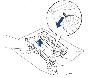
9. Turn the drum unit as shown in the illustration. Make sure that the drum unit gear (1) is on the left side.
