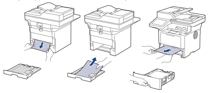
5. Remove paper that may have jammed under the machine due to static electricity.
