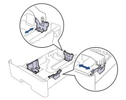
For Legal or Folio size paper, press the release button (1) in the bottom of the paper tray or the release lever (2) in the back of the tray, and then pull out the back of the paper tray. (Legal and Folio size paper are not available in some regions.)
