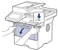
3. Remove the toner cartridge and drum unit assembly from the machine.
