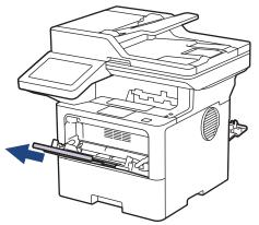
5. Slide the MP tray paper guides to fit the width of the envelopes that you are using.
