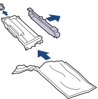
7. Hold the toner cartridge by the handle and shake it from left to right several times, as shown. Then push it firmly into the drum unit until it locks into place.
