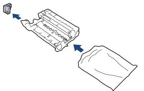
7. Push the toner cartridge firmly into the new drum unit until it locks into place.
