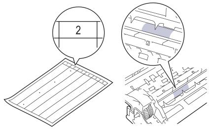
11. Turn the drum unit edge toward you while looking at the drum surface to find the mark.
