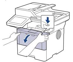
3. Remove the toner cartridge and drum unit assembly.
