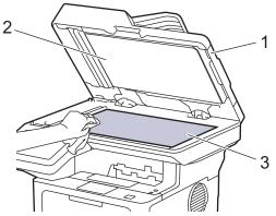
3. In the ADF unit, clean the white bar (1) and the scanner glass strip (2) underneath it with a soft lint-free cloth moistened with water.
