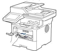
5. Load paper with the printing surface face up in the MP tray.
