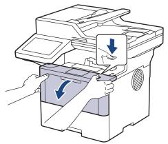
2. Remove the toner cartridge and drum unit assembly from the machine.
