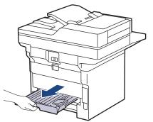
4. Pull the jammed paper out of the machine or out of the 2-sided tray.
