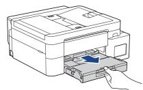
(DCP-T830DW/DCP-T835DW/MFC-T930DW/MFC-T935DW/MFC-T980DW) Lift the output paper tray cover (1).
