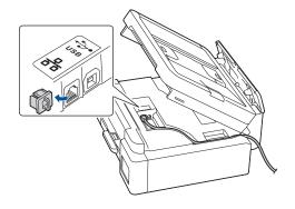
Carefully guide the cable through the cable channel and out the back of the machine.
