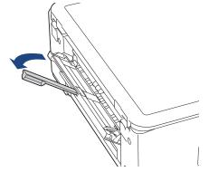
3. Slide the manual feed slot paper guides to fit the width of the paper you are using.
