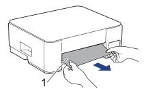
5. Squeeze both green levers together, and then lower the maintenance unit (1).
