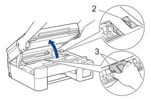
• If the paper is jammed under the print head, unplug the machine from the power source, and then move the print head to remove the paper.
