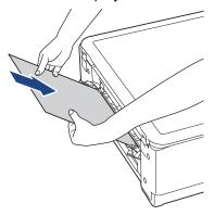
When loading an envelope, or a sheet of thick paper, push the media into the manual feed slot until you feel the paper feed rollers pull it.
