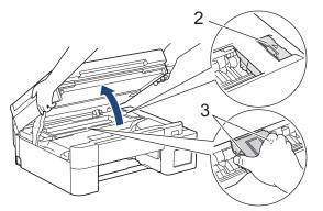
• If the paper is jammed under the print head, unplug the machine from the power source, and then move the print head to take out the paper.
