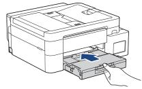
10. Pull out the paper support (1) until it locks into place, and then unfold the paper support flap (2).
