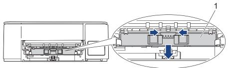
Clean the front and back sides of the Paper Feed Rollers (1) with a soft lint-free cloth moistened with water, using a side-to-side motion. After cleaning, wipe the rollers with a dry, soft lint-free cloth to remove all moisture.
