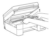
8. Move the print head (if needed) to take out any paper remaining in this area. Make sure scraps of paper are not left in the corners of the machine (1) and (2).
