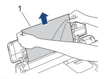
If you are having difficulty pulling paper out, push the release lever (1) toward the back of the machine, and then pull the paper.
