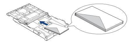
5. Gently press and slide the paper width guides (1) and paper length guide (2) to fit the size of the envelopes. Make sure the envelopes are flat in the tray.
