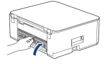
8. Put the paper support firmly back in the machine. Make sure you fit the paper support into the channels.
