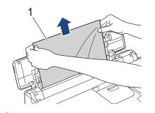
If you are having difficulty pulling the paper out, push the release lever (1) toward the back of the machine, and then pull the paper.
