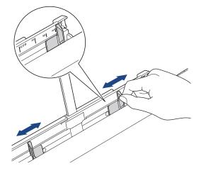
4. Load only one sheet of paper in the manual feed slot with the printing surface face up.
