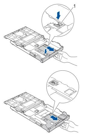
5. Gently press and slide the paper width guides (1) and the paper length guide (2) to fit the paper size.
