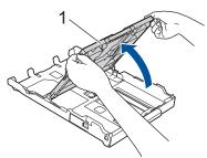
4. Press the square paper tray expansion button (1) and slide out the paper tray until the square paper tray expansion button locks into the square LGL hole.
