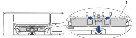
6. Clean the machine's printer platen (1) and the area around it, wiping off scattered ink with a dry, soft lint-free cloth.
