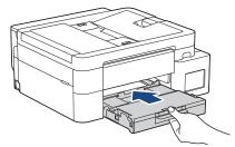
8. Pull out the paper support (1) until it locks into place, and then unfold the paper support flap (2).
