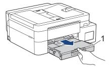
3. (DCP-T530DW/DCP-T535DW/DCP-T536DW/DCP-T730DW/DCP-T735DW/MFC-T580DW/MFC-T780DW) Lift the paper support (1), and then pull it at an angle completely out of the machine as shown by the arrow.
