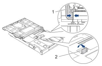
5. (DCP-T530DW/DCP-T535DW/DCP-T536DW/DCP-T730DW/DCP-T735DW/MFC-T580DW/MFC-T780DW) Gently press and slide the paper width guides (1) and then the paper length guide (2) to fit the paper size.
