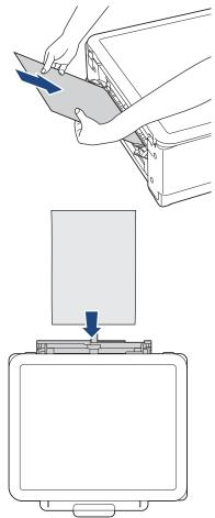
When using envelopes, load the envelopes with the printing surface **face up** and the flap on the left as shown in the illustration.
