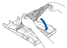
7. Load up to 20 sheets of photo paper with the printing surface face down.
