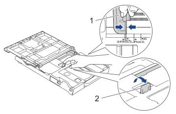
(DCP-T530DW/DCP-T535DW/DCP-T536DW/DCP-T580DW/DCP-T583DW/DCP-T730DW/DCP-T735DW/ DCP-T780DW) Gently press and slide the paper width guides (1) and then the paper length guide (2) to fit the paper size.
