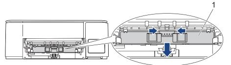
6. Clean the front and back sides of the Paper Feed Rollers (1) with a soft lint-free cloth moistened with water, using a side-to-side motion. After cleaning, wipe the rollers with a dry, soft lint-free cloth to remove all moisture.
