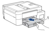
(DCP-T530DW/DCP-T535DW/DCP-T536DW/DCP-T580DW/DCP-T583DW/DCP-T730DW/DCP-T735DW/ DCP-T780DW) Lift the paper support (1), and then pull it at an angle completely out of the machine as shown by the arrow.
