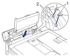
3. Pull the top of the MP tray cover slightly toward the front of the machine, and load paper in the MP tray with the printing surface face up.
