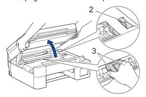
• If the paper is jammed under the print head, unplug the machine from the power source, and then move the print head to take out the paper.
