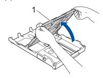
4. Load up to 10 envelopes in the paper tray with the printing surface **face down**. Loading more than 10 envelopes may cause paper jams.
