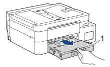
3. (DCP-T530DW/DCP-T535DW/DCP-T536DW/DCP-T580DW/DCP-T583DW/DCP-T730DW/DCP-T735DW/DCP-T780DW) Lift the paper support (1), and then pull it at an angle completely out of the machine as shown by the arrow.
