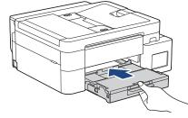
9. Pull out the paper support (1) until it locks into place, and then unfold the paper support flap (2).
