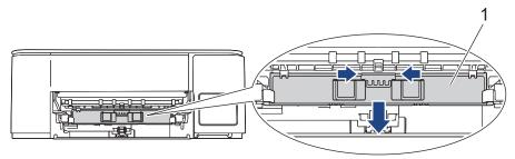
6. Clean the front and back sides of the Paper Feed Rollers (1) with a soft lint-free cloth moistened with water, using a side-to-side motion. After cleaning, wipe the rollers with a dry, soft lint-free cloth to remove all moisture.
