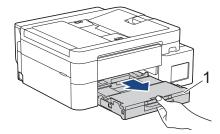
Lift the paper support (1), and then pull it at an angle completely out of the machine as shown by the arrow. (DCP-T530DW/DCP-T535DW/DCP-T536DW/DCP-T580DW/DCP-T730DW/DCP-T735DW/DCP-T730DW/DCP-T735DW/DCP-T780DW)
