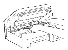
8. Move the print head (if needed) to take out any paper remaining in this area. Make sure scraps of paper are not left in the corners of the machine (1) and (2).
