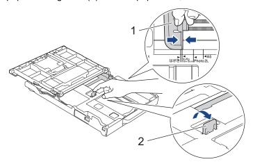
5. (DCP-T530DW/DCP-T535DW/DCP-T536DW/DCP-T580DW/DCP-T583DW/DCP-T730DW/DCP-T735DW/DCP-T780DW) Gently press and slide the paper width guides (1) and then the paper length guide (2) to fit the paper size.
