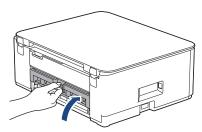
8. Put the paper support firmly back in the machine. Make sure you fit the paper support into the channels.
