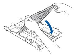
7. Load up to 20 sheets of photo paper with the printing surface face down.
