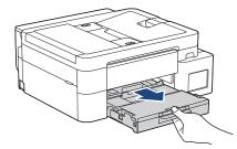
3. (DCP-T830DW/DCP-T835DW/MFC-T930DW/MFC-T935DW/MFC-T980DW) Lift the output paper tray cover (1).
