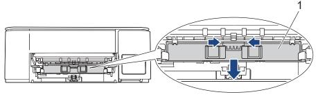
6. Clean the machine's printer platen (1) and the area around it, wiping off scattered ink with a dry, soft lint-free cloth.
