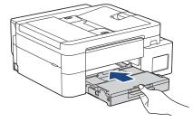
11. Pull out the paper support (1) until it locks into place, and then unfold the paper support flap (2).
