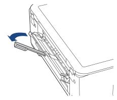
3. Slide the manual feed slot paper guides to fit the width of the paper you are using.
