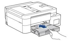
10. Pull out the paper support (1) until it locks into place, and then unfold the paper support flap (2).
