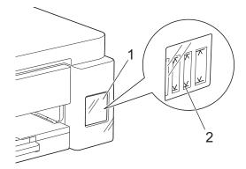
The ink below the lower line is necessary to prevent air from drying out and damaging the print head assembly. Refill the ink tank when the remaining ink level is at or below the lower line.
