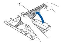
4. Press the square paper tray expansion button (1) and slide out the paper tray until the square paper tray expansion button locks into the square LGL hole.
