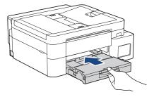
11. Pull out the paper support (1) until it locks into place, and then unfold the paper support flap (2).
