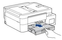
12. Pull out the paper support (1) until it locks into place, and then unfold the paper support flap (2).
