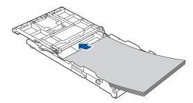
Make sure the paper is flat in the tray and the paper length guide (1) touches the edges of the paper.
