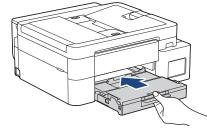
6. Pull out the paper support (1) until it locks into place, and then unfold the paper support flap (2).
