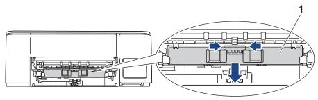
6. Clean the machine's printer platen (1) and the area around it, wiping off scattered ink with a dry, soft lint-free cloth.
