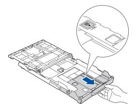
5. Gently press and slide the paper width guides (1) and the paper length guide (2) to fit the paper size.
