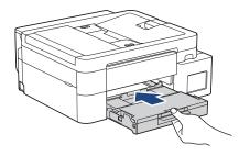
14. Pull out the paper support (1) until it locks into place, and then unfold the paper support flap (2).
