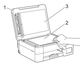
3. In the ADF unit, clean the white bar (1) and the glass strip (2) with a lint-free cloth moistened with water. (ADF models only)
