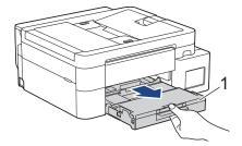
3. (DCP-T530DW/DCP-T535DW/DCP-T536DW/DCP-T730DW/DCP-T735DW) Lift the paper support (1), and then pull it at an angle completely out of the machine as shown by the arrow.
