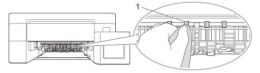
5. Lift the flap (2), and then clean the back side of the Paper Feed Rollers (1) with a soft lint-free cloth moistened with water. After cleaning, wipe the rollers with a dry, soft lint-free cloth to remove all moisture.
