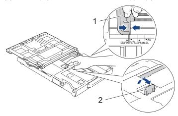
5. (DCP-T530DW/DCP-T535DW/DCP-T536DW/DCP-T730DW/DCP-T735DW) Gently press and slide the paper width guides (1) and then the paper length guide (2) to fit the paper size.
