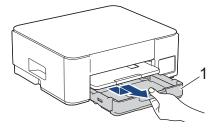
4. Lift the paper support (1), and then pull it at an angle completely out of the machine as shown by the arrow.
