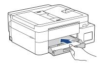
11. Pull out the paper support (1) until it locks into place, and then unfold the paper support flap (2).
