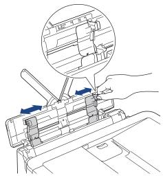
4. Fan the stack of paper well to avoid paper jams and misfeeds.
