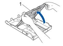
4. (DCP-T830DW/DCP-T835DW/MFC-T930DW/MFC-T935DW) Gently press and slide the paper width guides (1) to fit the paper size, and then lift the stopper (2).
