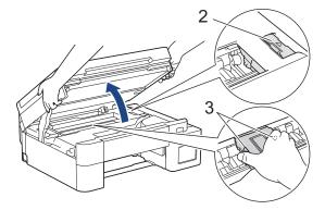
• If the paper is jammed under the print head, unplug the machine from the power source, and then move the print head to remove the paper.
