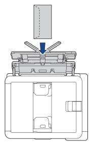
If you are having difficulty loading paper in the MP tray, push the release lever (1) towards the back of the machine, and then load the paper.
