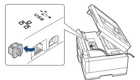
Carefully guide the cable through the cable channel and out the back of the machine.
