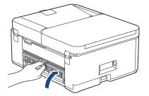
7. Put the paper support firmly back in the machine. Make sure you fit the paper support into the channels.
