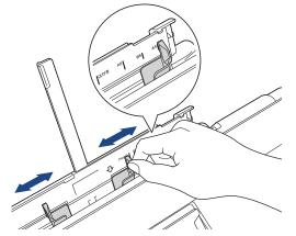
4. Load only **one sheet of paper** in the manual feed slot with the printing surface **face up**.
