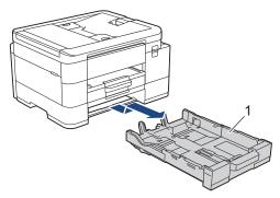
4. Clean the paper pick-up rollers for Tray #2 (1) with a soft lint-free cloth moistened with water. Slowly turn the rollers so that the whole surface is cleaned. After cleaning, wipe the rollers with a dry, soft lint-free cloth to remove all moisture.
