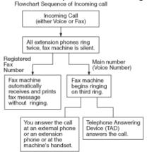
After you have set the FaxAbility feature to on, the receive mode is set to [Manual] automatically. Unless you have a TAD or Voice Mail set up on the FaxAbility number, Manual mode means you must answer all the call yourself. You can not change the receive mode to the other mode while the FaxAbility is set to on. When FaxAbility is on, the LCD will show [D/R] as the Receive Mode.
