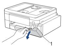
2. Press the lock release lever to release the ink cartridge colour indicated on the LCD and remove the ink cartridge from the machine, as shown in the illustration.
