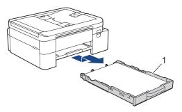
(MFC-J4555DW) If your LCD error message was [Jam Tray2], also pull Tray #2 (2) completely out of the machine as shown by the arrow.
