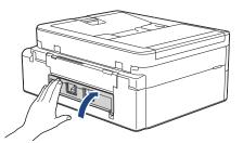
8. If your LCD error message was [Jam Rear], put the paper support firmly back in the machine. Make sure you fit the paper support into the channels.
