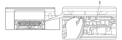
6. Lift the flap (2), and then clean the back side of the Paper Feed Rollers (1) with a soft lint-free cloth moistened with water. After cleaning, wipe the rollers with a dry, soft lint-free cloth to remove all moisture.
