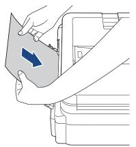
When loading an envelope, or a sheet of thick paper, push the media into the manual feed slot until you feel the paper feed rollers pull it.
