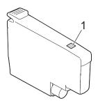
(MFC-J4350DW/MFC-J4355DW/MFC-J4555DW) Quickly shake just the **black** ink cartridge horizontally 15 times as shown, before inserting it into the machine.
