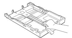
6. Wipe the outside of the paper support with a dry, lint-free cloth to remove dust.
