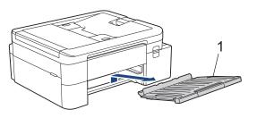
Depending on the paper size, it is easier to remove the jammed paper from the front of the machine rather than from the back of the machine.
