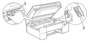
• If the paper is jammed under the print head, unplug the machine from the power source, and then move the print head to remove the paper.
