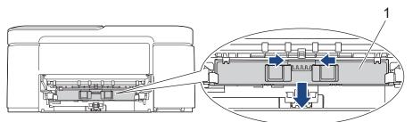
6. Clean the front and back sides of the Paper Feed Rollers (1) with a soft lint-free cloth moistened with water, using a side-to-side motion. After cleaning, wipe the rollers with a dry, soft lint-free cloth to remove all moisture.
