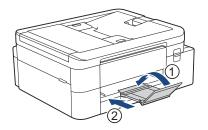
2. Pull the paper tray completely out of the machine.
