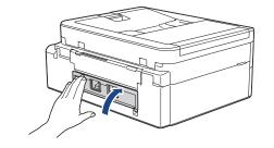
8. Put the paper support firmly back in the machine. Make sure you fit the paper support into the channels.
