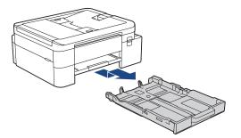
3. Load up to 10 envelopes in the paper tray with the printing surface **face down**. Loading more than 10 envelopes may cause paper jams.
