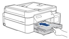
14. While holding the paper tray in the machine, pull out the paper support (1) until it locks into place, and then unfold the paper support flap (2).
