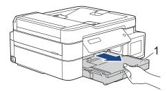
4. Clean the front side of the Paper Feed Rollers (1) with a soft lint-free cloth moistened with water, using a side-to-side motion. After cleaning, wipe the rollers with a dry, soft lint-free cloth to remove all moisture.
