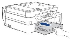
11. While holding the paper tray in the machine, pull out the paper support (1) until it locks into place, and then unfold the paper support flap (2).
