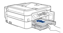
6. While holding the paper tray in the machine, pull out the paper support (1) until it locks into place, and then unfold the paper support flap (2).
