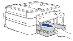
7. Pull out the paper support (1) until it locks into place, and then unfold the paper support flap (2).
