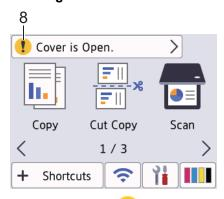
The warning icon • appears when there is an error or maintenance message; press • to view the details, and then press × to return to the Home screen.
