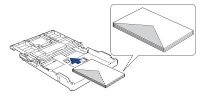
5. Gently press and slide the paper width guides (1) and paper length guide (2) to fit the size of the envelopes. Make sure the envelopes are flat in the tray.
