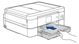
6. Pull out the paper support (1) until it locks into place, and then unfold the paper support flap (2).
