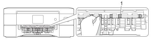
5. Lift the flap (2), and then clean the back side of the Paper Feed Rollers (1) with a soft lint-free cloth moistened with water. After cleaning, wipe the rollers with a dry, soft lint-free cloth to remove all moisture.
