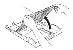
4. Gently press and slide the paper width guides (1) to fit the paper size, and then lift the stopper (2).
