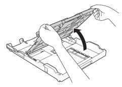
5. Wipe the inside and the outside of the paper tray with a dry, lint-free cloth to remove dust.
