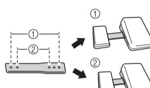
The pedal spacing can be adjusted depending on the screw holes used in the mounting plate. The pedal spacing is the widest when the pedals are attached using the outermost screw holes (1); the pedal spacing is the narrowest when they are attached using the innermost screw holes (2).
