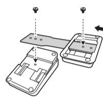
Align the wide side of the mounting plate with the notch in the bottom of the main foot controller, and then secure them together with a screw. Feed the other side of the mounting plate into the notch on the bottom of the side pedal, and then secure them together with a screw.
