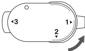
You can install/remove the presser foot holder, needle clamp screw.
