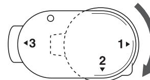
The multi-purpose screwdriver can be positioned over the screw on the embroidery frame to tighten the screw after hooping the fabric or when removing the fabric.
