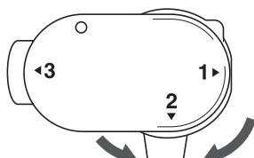
You can install/remove the needle plate.
