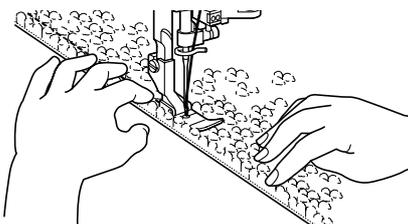
Pull the upper thread under the presser foot through the slit in the foot.
