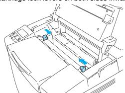
4 Remove the OPC belt cartridge from the printer.
