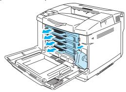
9 To avoid spreading the toner, plug the supplied protective sponge into the area of the printer as shown in the illustration.
