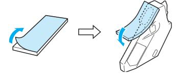
11 Fit an orange protective cover to each of the toner cartridges. Secure it with tape.
