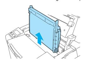
Place the OPC belt cartridge into the plastic bag, and then put it in the original box.
