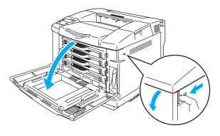
Pull out all the toner cartridges and waste toner pack from the printer.
