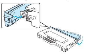
**12** Put all the toner cartridges and waste toner pack into the printer.
