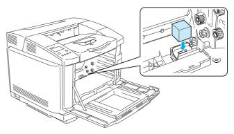
10 Remove the tape from the supplied protective sponge, and then cover the opening of the waste toner pack as shown in the illustration.
